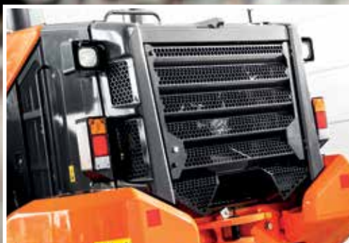
New rear grille protects radiator compartment.
