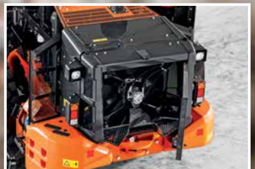
Durable radiators are corrosion resistant.
