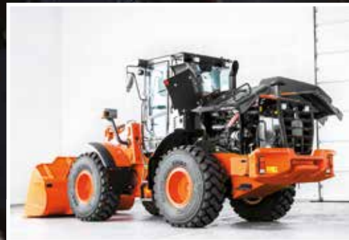
Easy access for maintenance from ground level.
