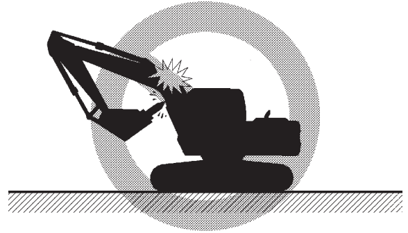
Warning about Touching the Boom
