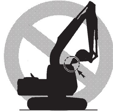
Warning about Rolling Too Far with the Bucket
