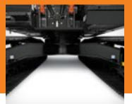
Thick-plate single-sheet mainframe, box-section track frames and industry exclusive double-seal swing bearing deliver rock-solid durability.
