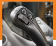
Ergonomically correct shortthrow pilot levers provide smooth, precise control with less effort. Standard sliding switch provides proportional speed control, giving you full command from your fingertips. Optional cab and right-side boom lights provide extra illumination to extend your production.
