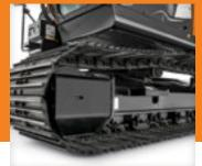
With large idlers, rollers and strutted track links, the sealed and lubricated undercarriage is built for the long haul.
