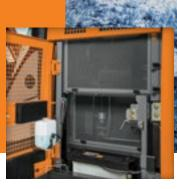
Ground-level-accessible coolers with easily removed pre-cleaner screens help prevent trash from plugging up the cores – helping maintain cool-running efficiency.
