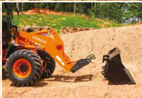
Universal Quick Couple allows seamless transition (ZW80-5b).
